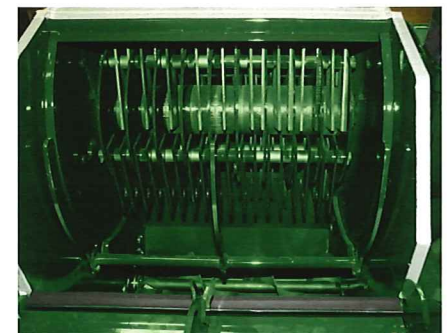
72 hardened 4 way reversible hammers for faster grinding speeds and more consistent grinds.
